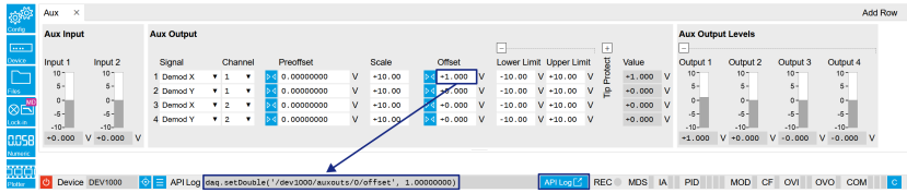
Figure 71: When a device's configuration is modified in the LabOne User Interface, the Status Bar displays the equivalent command to perform the same configuration via a LabOne programming interface. Here, the MATLAB code to modify auxiliary output 1's offset value is provided. When "Show Log" is clicked the entire configuration history is displayed in a new browser tab.
